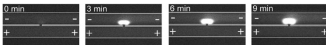
Fig. 9 Visualization of green fluorescent protein (GFP) focusing at the enrichment side nanochannel interface. The model presented here predicts that this analyte should focus on a propagating enrichment shock, not at this interface. We hypothesize the discrepancy may be due to the low field values used or to our uncertainty in GFP mobility at these conditions. Reprinted with permission from Schoch et al. 16
