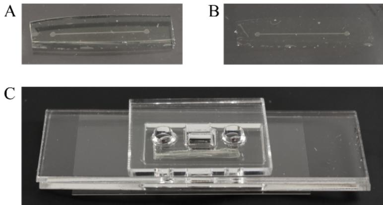
**Figure 2: Images of completed MY133-V2000 devices.** (A) The edges of the MY133-V2000 device are distinctly visible in air. (B) When submerged in water, the edges of the same MY133-V2000 device disappear because of the close match in refractive indices. (C) This photograph shows a finished device with an acrylic holder. [Please click here to view a larger version of this figure.](#)
