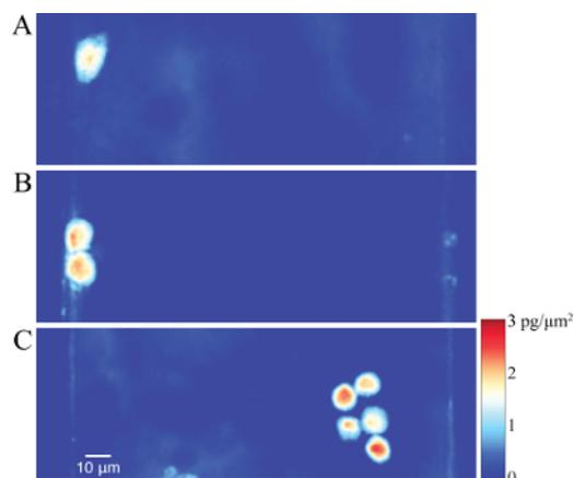
**Figure 3: Cell mass can be precisely quantified near microchannel structures.** Measurements of the cell mass of freshly seeded MCF7 cells in the MY133-V2000 microchannel show no artifacts due to phase wrapping near (A and B) the wall or (C) the center of the channel. These artifacts are avoided in the MY133-V2000 channel because of the closely matched refractive indices of the channel material and the cell culture media. [Please click here to view a larger version of this figure.](#)
